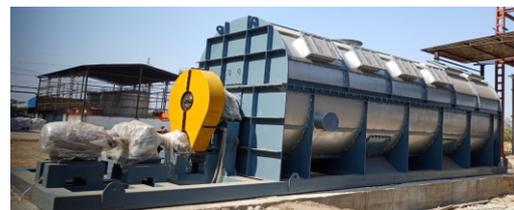
The absence of a rotating shell eliminates the need for complicated mechanical components, such as tires, trunnion rollers. This simplification results in a more compact and efficient design, reducing maintenance requirements and enhancing overall reliability.
